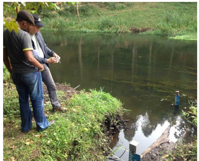
Reviewing gauge data for the Kaku River in Uganda. Read twice daily, these river gauges provide the hydrology data critical to a bankable hydropower project.
