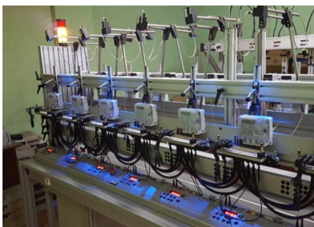
Single-phase meters being tested on a partially functioning meter test bench in EEU.
