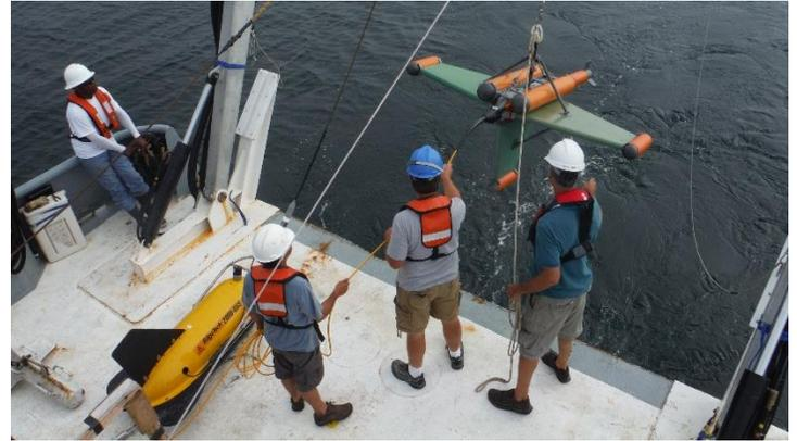
The 4-sensor MGA being deployed for a cable route survey
