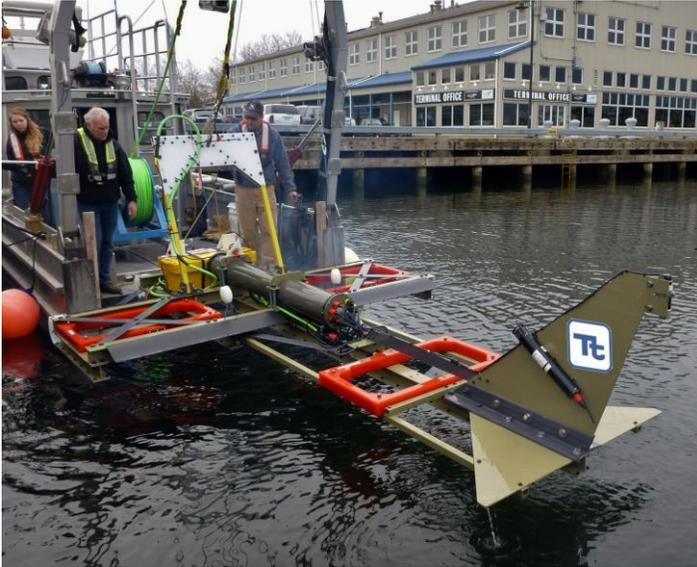
Tetra Tech has developed, refined, and deployed custom underwater MEC/UXO detection systems for more than a decade.
