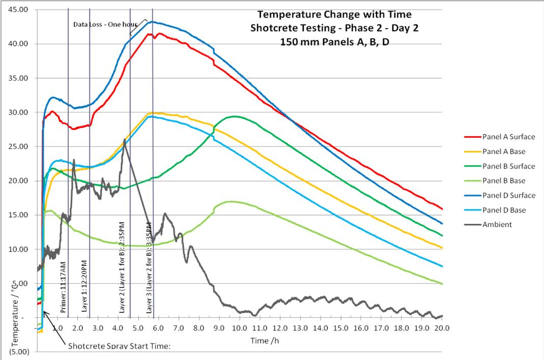
Figure 2: Temperature profiles of shotcrete on frozen rock with membrane, (Ouellet, 2011).
