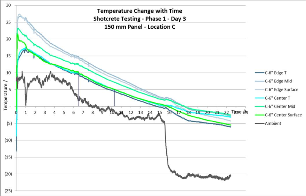
Figure 1: Temperature profiles of shotcrete on frozen rock, (Ouellet, 2011).
