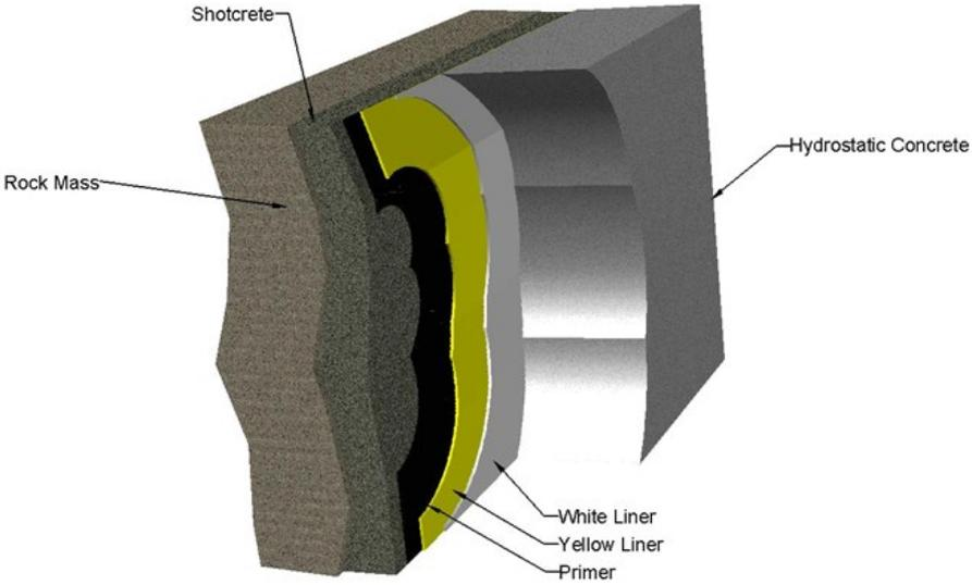
**Figure 3: Composite liner concept with sprayed on membrane.**
