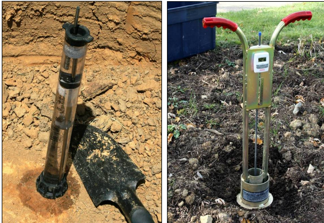
Figure 3 – Infiltration testing at 2-foot depth (left) and on surface of completed garden (right)
