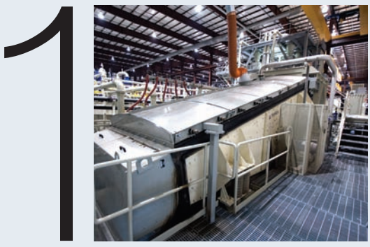
1 Screening. The first stop for incoming slurry is the scalping screen, which removes debris larger than 6 mm in diameter. Items removed include wood chips, bottles and large rocks.
